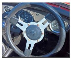
The steering wheel pictured was found by a scrutineer at a hill climb event last month. Of the six bolts that should be holding the steering wheel to the boss, one bolt was completely missing, one bolt had no nut (the screw fell out upon
