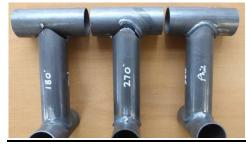
From the test result it would appear there is a direct correlation between weld coverage and achievable load. i.e.:
